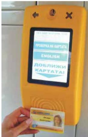
In trams and trolleybuses, the fare is collected from the card at special devices, validators:
